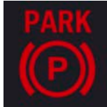
F10 Indicator light, parking brake engaged display
